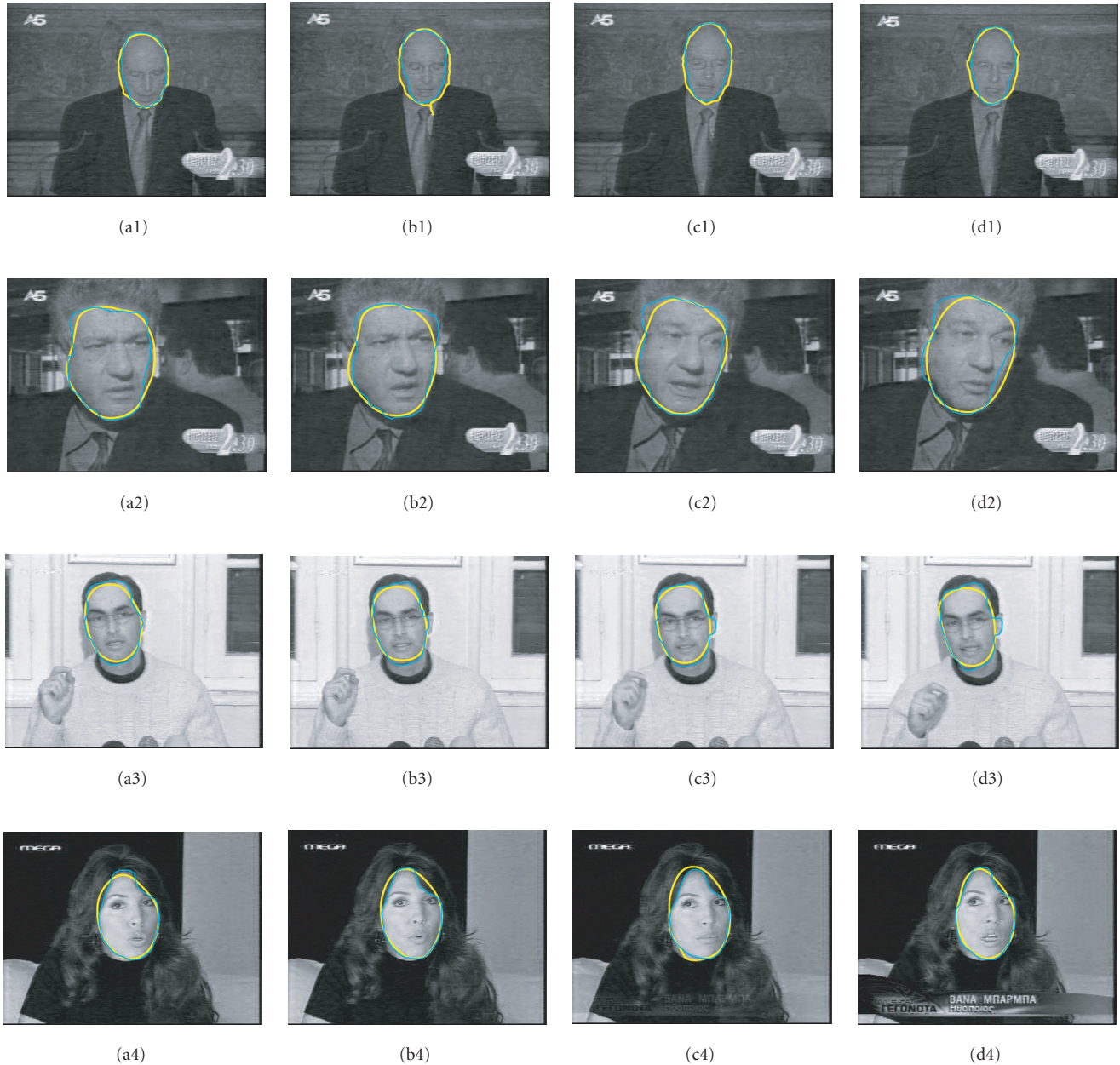
FIGURE 17: Face tracking results of the proposed method after applying the model-based (shape prior) term: the final contours are illustrated in bold curves, whereas the results obtained without the shape prior (Figure 16), are shown in soft curves.
