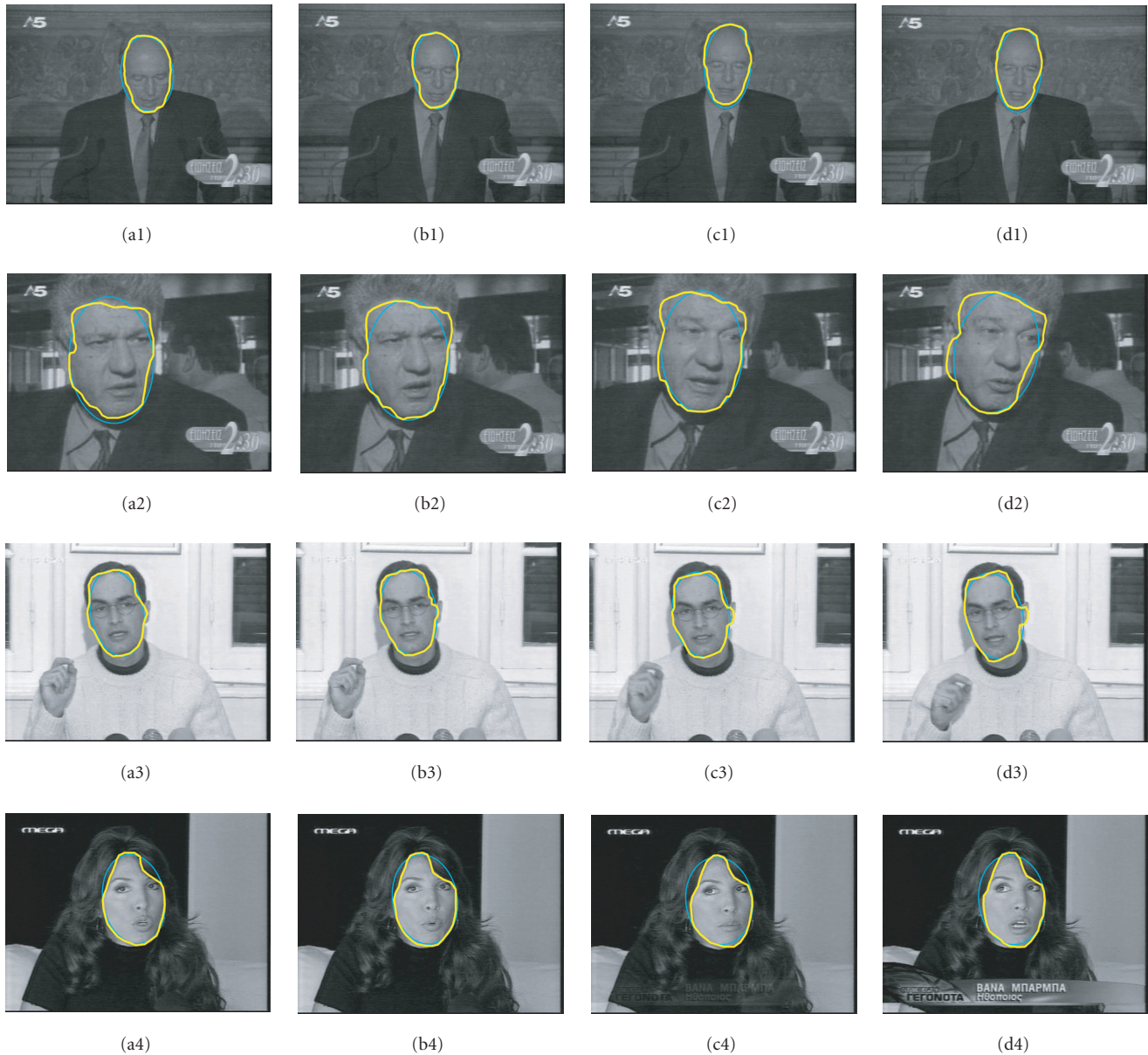
FIGURE 16: Face tracking results of the proposed rule-based method without applying the model-based term: the final results (contours) are illustrated in bold curves, whereas the shape prior (ellipse), to be further applied (Figure 17), is shown in soft curves.
