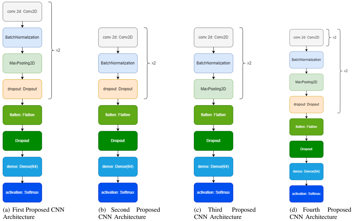
Fig. 1. Detailed diagrams of the four proposed CNN architectures, each showcasing layer configurations and operational flows to optimize garbage classification.
